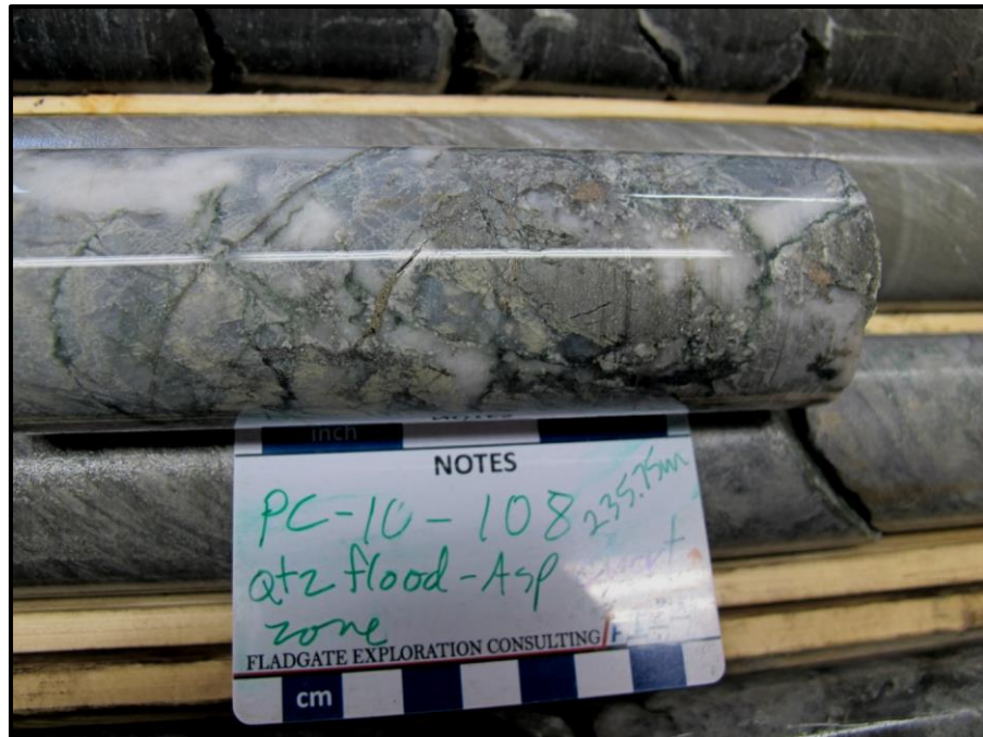
Figure 7.27 Semi-massive Arsenopyrite in Quartz-Flooded Chert-Rich Iron Formation, Central Pat East Zone In Hole PC-10-108
