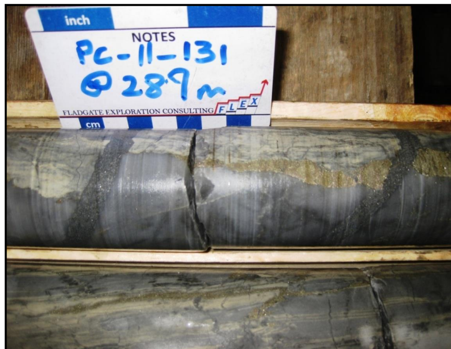
Figure 7.31 High Angle Arsenopyrite Veinlets Cutting Low Angle Bedding in Chert-Rich Iron Formation Central Pat East Zone in Hole PC-11-131
