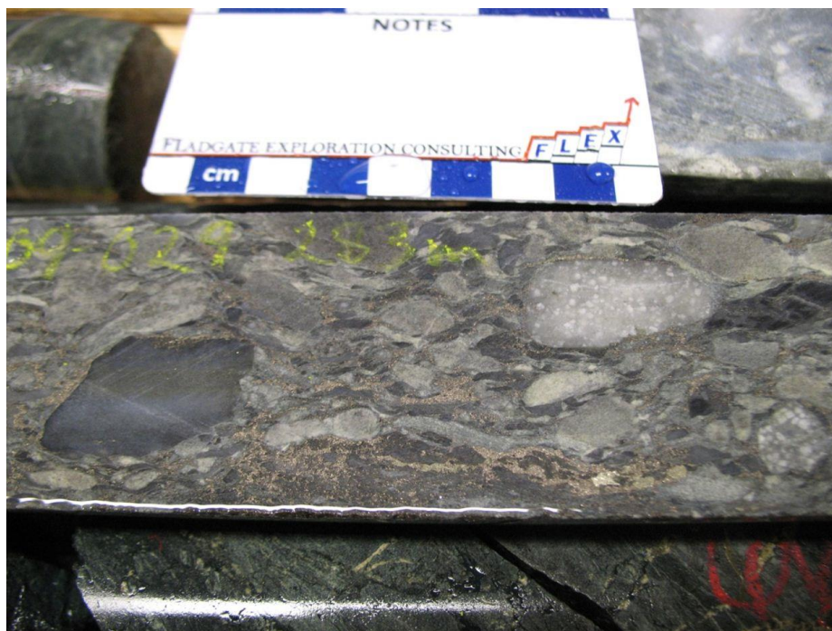
Figure 7.8 Polymictic Temiskaming-like Conglomerate, Shaft 3 Area Hole PC-09-029
