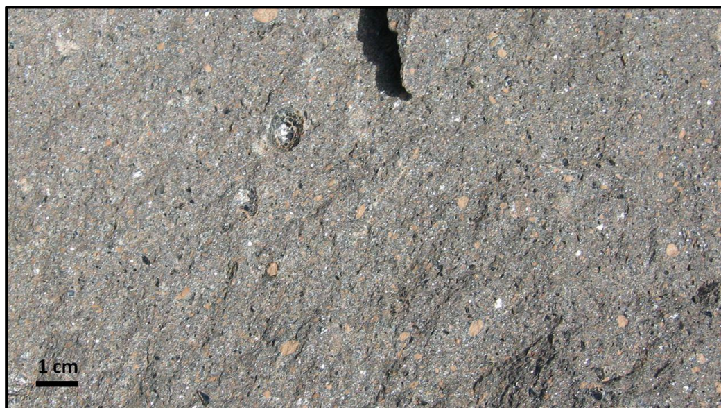
Figure 7.12 Carbonate Altered Lamprophyre Dyke, No. 1 Vein Surface Stockpile
