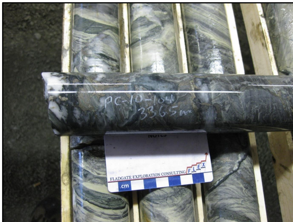
Figure 7.25 Gold-Bearing Patchy Quartz Veining and Disseminated Pyrite-Pyrrhotite Mineralization from the Kawinogans Zone In Hole PC-10-090
