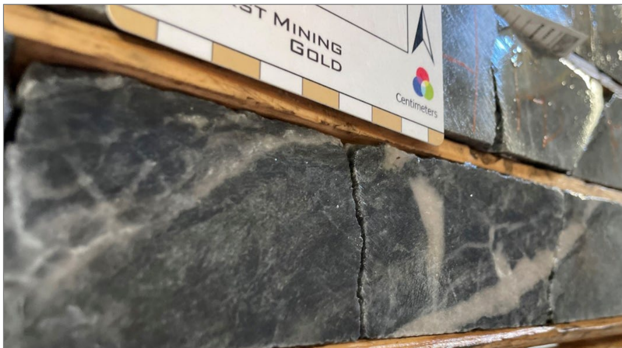
Figure 2: Representative core sample from the North Zone, highlighting alteration and veining.
