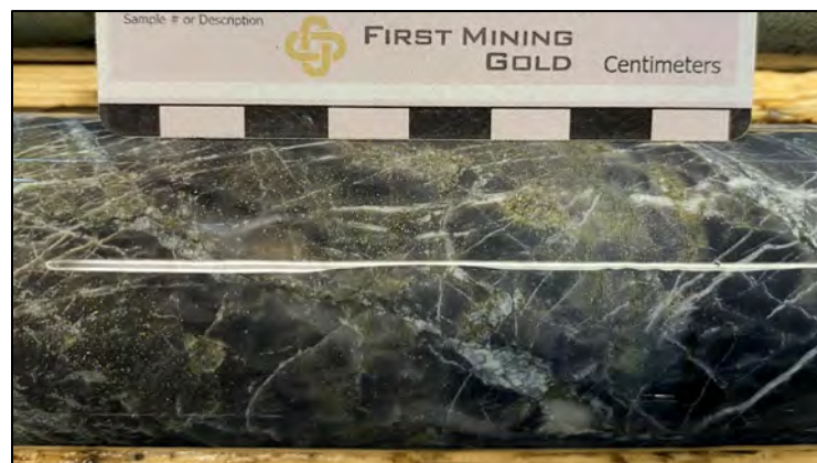
Aiguille: Dark smokey quartz vein with disseminated pyrite mineralization in DUP24-041
