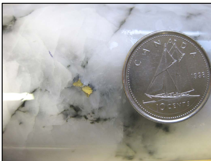
Figure 9.3 Visible Gold in Quartz with Tourmaline-filled Fractures, No. 19 Vein In Hole PC-09-052A
