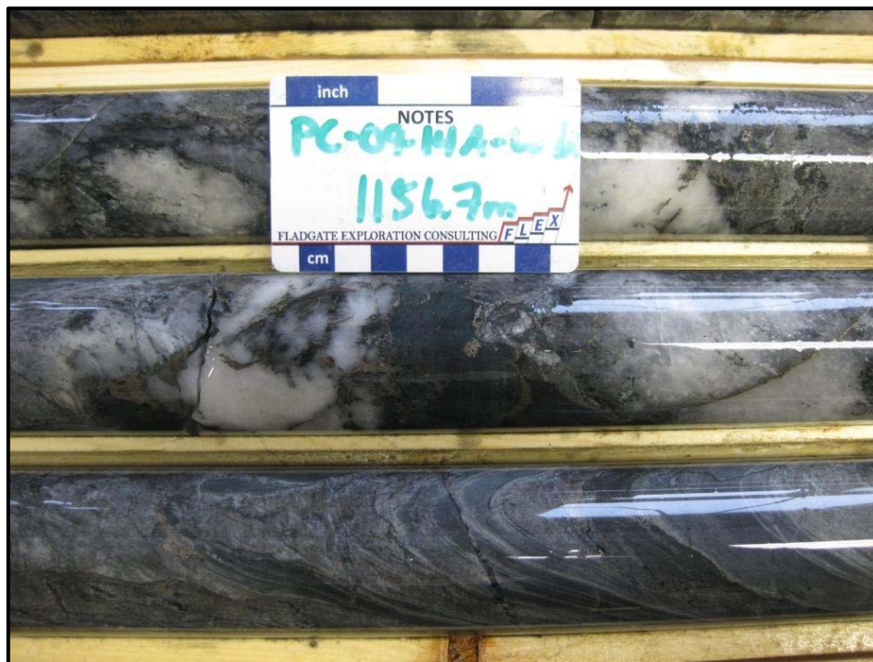
Figure 9.6 Gold-Bearing Patchy Quartz Veining and Disseminated Pyrite-Pyrrhotite Mineralization From the No. 5 BIF Zone in Hole PC-09-014A-W04
