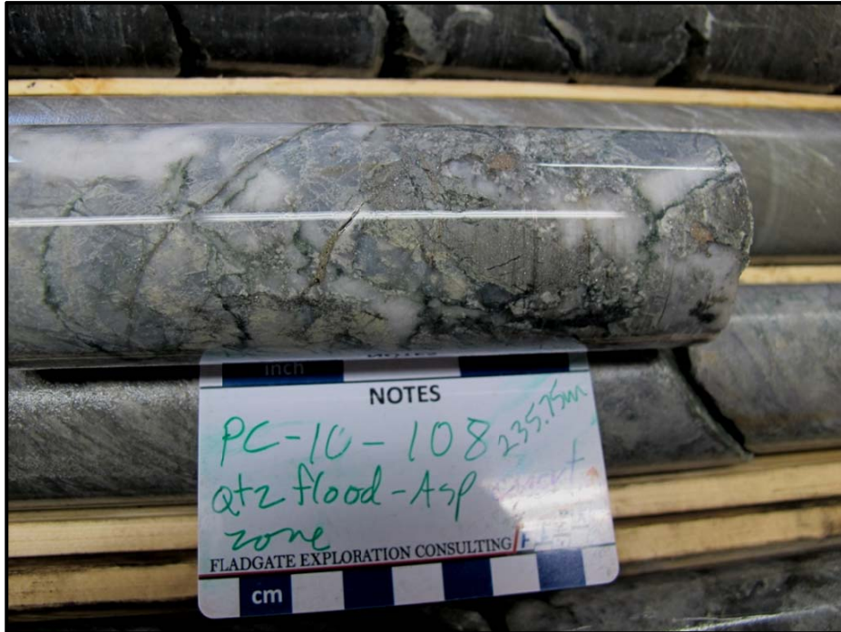
Figure 9.10 Photomicrograph of Arsenopyrite Associated Gold Mineralization, Central Pat East Zone In Hole PC-10-108
