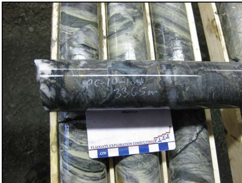
Figure 9.7 Gold-Bearing Patchy Quartz Veining and Disseminated Pyrite-Pyrrhotite Mineralization from the Kawinogans Zone In Hole PC-10-090
