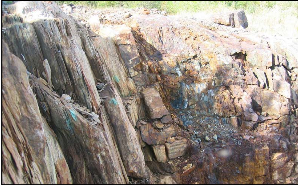
Figure 7.16 D2 Shear Zone Containing No. 5 Vein, West End of No. 5 Bulk Sample Pit
